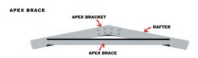
Note: Under NO circumstances are the Apex Braces to be fitted to the lips of the C Section.
