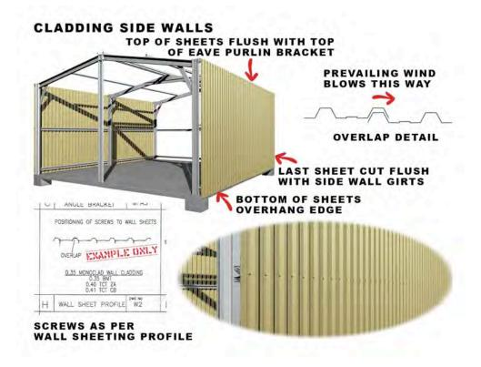
If an opening (Personal Access Door, Roller Door, Glass Sliding Door or Window) is to be installed on the side wall allow the standard overlap on wall cladding and leave out the wall sheeting where the door or window is to be positioned until all other sheets are screwed into position. Install the sheets above the door or window once the height of the door has been established. Refer to the relevant chapter(s) for more details:
