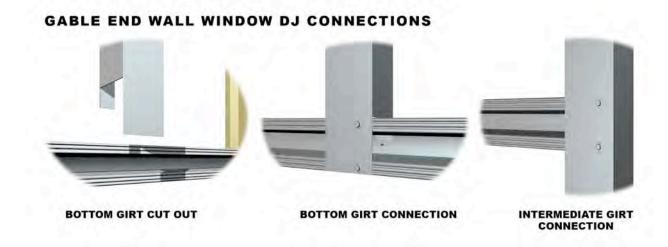
Fit L/H and R/H side wall door jambs and screw the two upright (uncut) legs to both sides of the GABLE END WALL GIRT ABOVE or RAFTER using Framing Screws. Plumb the jambs, and screw the bottom upright (uncut) legs to the GABLE END WALL GIRT BELOW. If the Jamb sits on the slab then drill holes in the base cleat and anchor bolt into position. Fix the door jambs at intersection of any girt(s) which were cut off.
