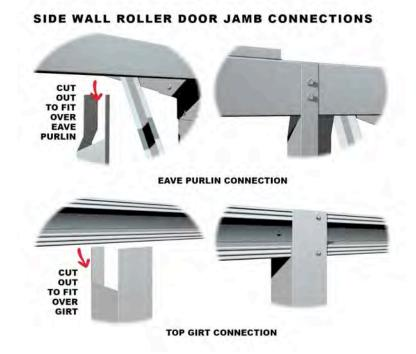
Ensure the jambs are plumb, then fix a base cleat to the bottom of each door jamb (with offset as per manufacturers installation material) and anchor bolt into position. Fix the door jambs at each intersection of girts which were cut off.
